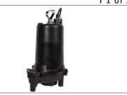
A.Y. McDonald's 1 & 2 HP grinder pumps have a 1 1/4" vertical discharge (optional 2" adapter available), and can grind up to 3" solids, and be installed on a rail system or with the supplied legs. Suitable for use in residential developments, commercial developments and wastewater applications.
