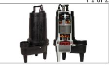
A.Y. McDonald's 1/2 HP Sewage Pumps handle up to 2" solids with a 2" discharge. Applications include basements, dewatering, septic systems, sewage lift stations, add-a-baths and truck docks for applications.
