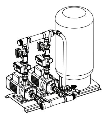
The DuraMAC<sup>™</sup> Dual-Mode Commercial Booster System can be installed in multiple pump configurations to increase the flow capacity. In this arraignment one pump will be the Lead pump and the other pump will be the Lag pump.
