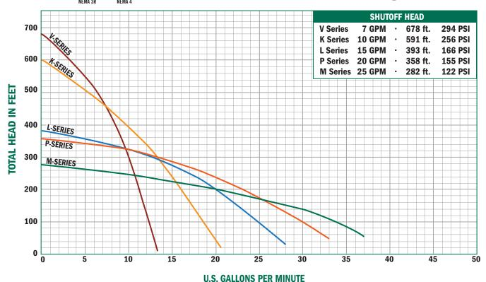
NOTE: Performance shown does not include friction loss in drop pipe (for flow rates above 25 GPM, larger drop pipe is recommended.)
