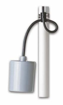
This pump switch is designed to directly control pumps up to 0.5 HP at 120 VAC in non-potable water and sewage applications. The switch is not sensitive to turbulence, allowing it to be used in both calm and turbulent applications. It can be wired to work in either pump down (normally open) or pump up (normally closed) applications.
