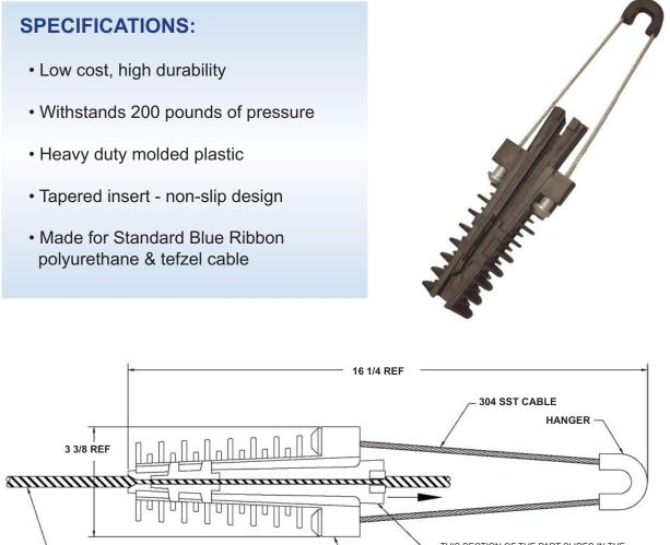
THIS SECTION OF THE PART SLIDES IN THE DIRECTION OF THE ARROW TO RELEASE THE ELECTRIC CABLE. THEN SLIDES IN OPPOSITE DIRECTION OF THE ARROW TO CLAMP DOWN ON THE ELECTRIC CABLE.
