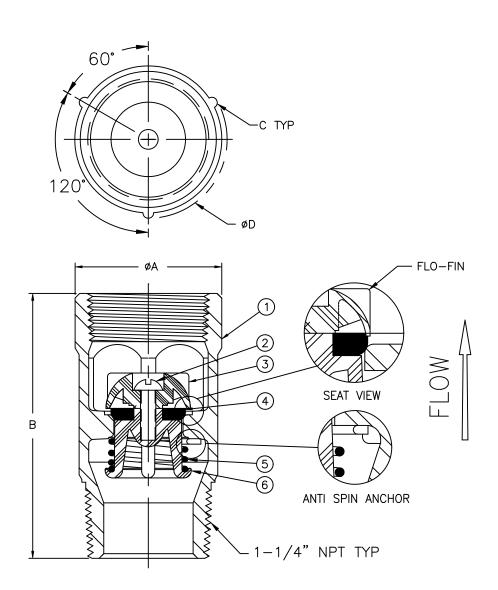
Max Temp 180°F (82°C) Max Pressure 400psi (28bar)
