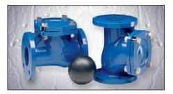
Model 408, 408<sup>2</sup> & 408FB A favorite and proven valve Model in the submersible water and wastewater industry for decades. The 408 features a clean-out port permitting access to the inside of the valve without removal from the pipe line. Flanged ANSI 125 connections. Model 408FB is equipped with a "floating" rather than a "sinking" ball to prevent backflow from drains.
