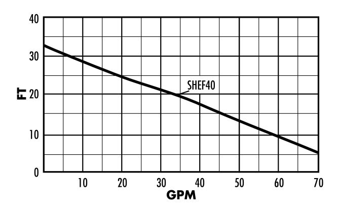
The curves reflect maximum performance characteristics without exceeding full load (Nameplate) horsepower. All pumps have a service factor of 1.2. Operation is recommended in the bounded area with operational point within the curve limit. Performance curves are based on actual tests with clear water at 70° F. and 1280 feet site elevation.
