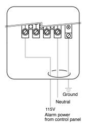
The model AHW is wired directly to the 115 VAC remote alarm connection of the control panel. This connection is identified on the panel wiring diagram as shown below.
