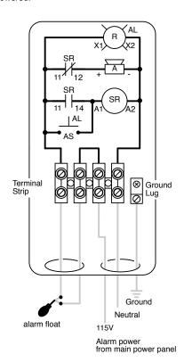
To insure alarm operation during a pump fault. power this alarm from a different power source than the pump, in pump tank systems.
