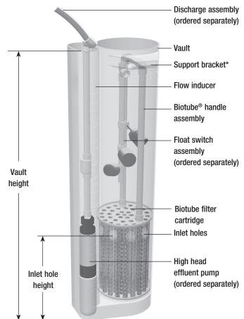
\* The distance between the top of the vault and the bottom of the support bracket is 3 inches (76 mm), so the vault extends that far above the opening on which the support pipes rest.
