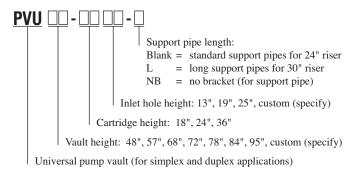
Orenco's Biotube Pump Vault is available in standard and customized configurations. Contact Orenco or your nearest distributor for sizing recommendations.
