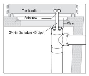
Cartridge handles can be extended for easier access.
