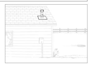
Carbon filters are often installed on roof vents to control odors. Use proper safety equipment and practices when working on roofs.
