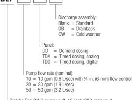
Biotube EasyPak<sup>™</sup> pump vault, 15-inch (380-mm) vault
