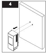
Remove old controller from the wall.
