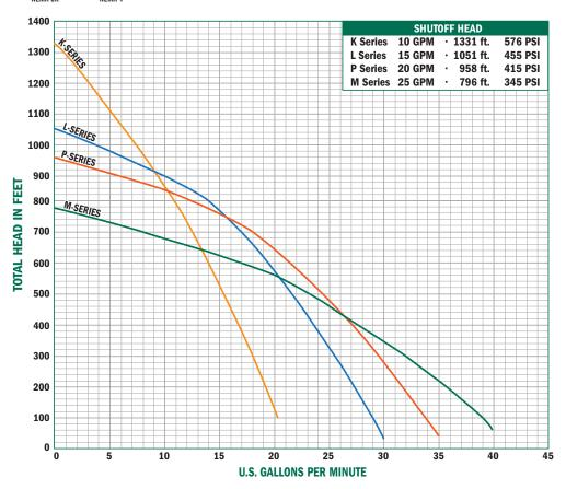
NOTE: Performance shown does not include friction loss in drop pipe (for flow rates above 25 GPM, larger drop pipe is recommended.)
