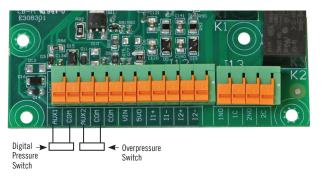
Connection Diagram for Digital Pressure Switch. Digital pressure switch connected to AUX1 and COM, overpressure switch connected to AUX2 and COM.
