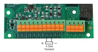
Connection Diagram for 4-20 mA Analog Transducer
