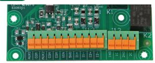
AutoDRIVES are equipped with Control Terminals that allow a number of control functions
