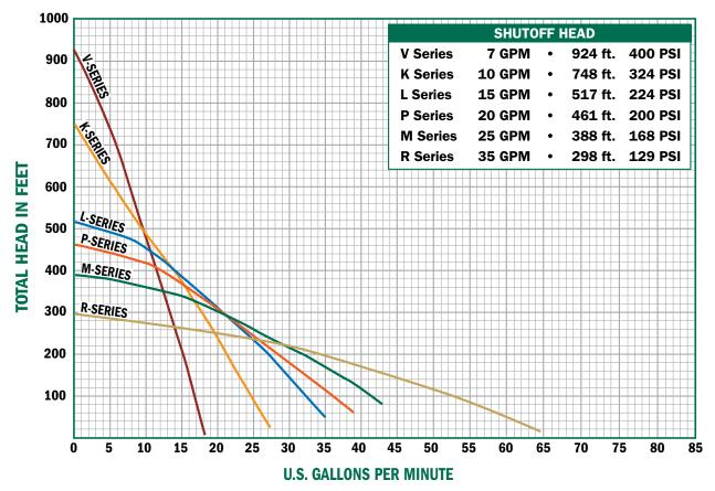
NOTE: Performance shown does not include friction loss in drop pipe (for flow rates above 25 GPM, larger drop pipe is recommended.)
