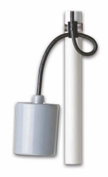
This pump switch is designed to directly control pumps up to 0.75 HP at 120 VAC and 2 HP at 230 VAC in non-potable water and sewage applications. The switch is not sensitive to turbulence, allowing it to be used in both calm and turbulent applications.
