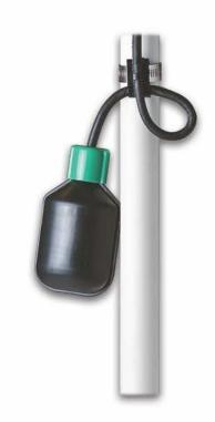
This control switch is used to accurately monitor high (normally open) or low (normally closed) liquid levels to activate pump control panels and alarms in water and sewage applications. It features a green colored cap for easy identification of SPDT control switch. This switch can be wired to work in either normally open or normally closed applications.
