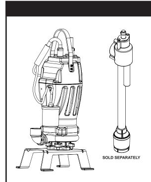
Series: ZOGV-AU 2HP, 3450RPM, 60Hz with Level Control
