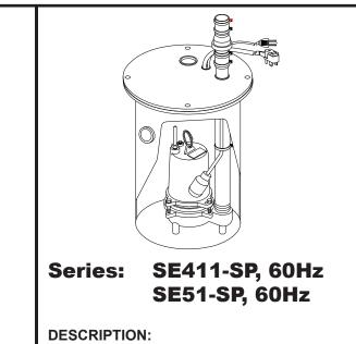
SIMPLEX SYSTEMS (ONE PUMP) ARE GOOD FOR RESI-DENCES AND SMALL INDUSTRIAL SEWAGE OR SUMP APPLICATIONS. THEY ARE DESIGNED TO HANDLE WASTES FROM LAVATORIES, LAUNDRY TUBS, FLOOR DRAINS, WATER CLOSETS, ETC., AND WILL PUSH THE WATER FROM BELOW GROUND UP TO WHERE NORMAL DRAINAGE WILL HANDLE IT.
