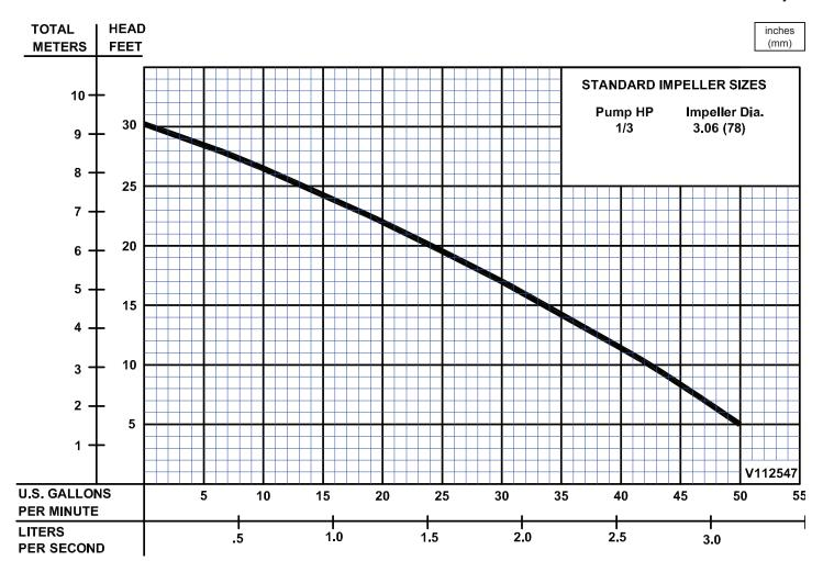
Testing is performed with water, specific gravity 1.0 @  $68^{\circ}$  F @ (20°C), other fluids may vary performance
