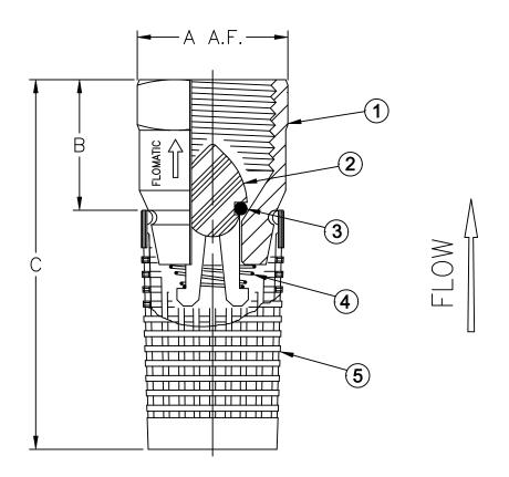
Open Area: 30-40% Max Temp 180°F (82°C) Max Pressure 150psi (10bar)
