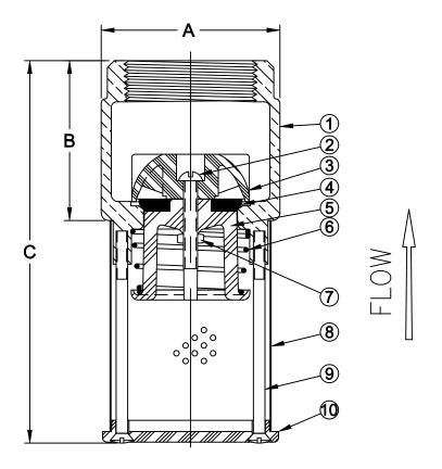
Open Area: 35-50% Max Temp 180°F (82°C) Max Pressure 250psi (18bar)
