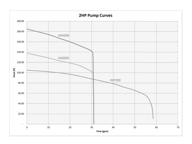
The curves reflect maximum performance characteristics without exceeding full load (Nameplate) horsepower. All pumps have a service factor of 1.2. Operation is recommended in the bounded area with operational point within the curve limit. Performance curves are based on actual tests with clear water at 70° F and 1280 feet site elevation.
