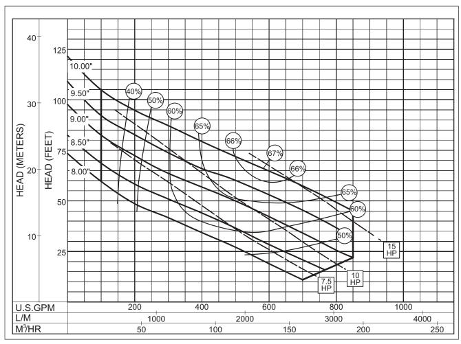
The curves reflect maximum performance characteristics without exceeding full load (Nameplate) horsepower. All pumps have a service factor of 1.2. Operation is recommended in the bounded area with operational point within the curve limit. Performance curves are based on actual tests with clear water at  $70^{\circ}$  F. and 1280 feet site elevation.
