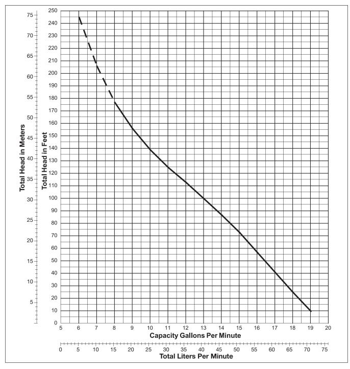
The curves reflect maximum performance characteristics without exceeding full load (Nameplate) horsepower. All pumps have a service factor of 1.0. Operation is recommended in the bounded area with operational point within the curve limit. Performance curves are based on actual tests with clear water at 70° F. and 1280 feet site elevation.
