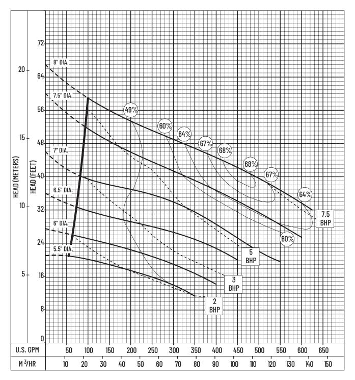
The curves reflect maximum performance characteristics without exceeding full load (Nameplate) horsepower. All pumps have a service factor of 1.2. Operation is recommended in the bounded area with operational point within the curve limit. Performance curves are based on actual tests with clear water at  $70^{\circ}$  F. and 1280 feet site elevation.
