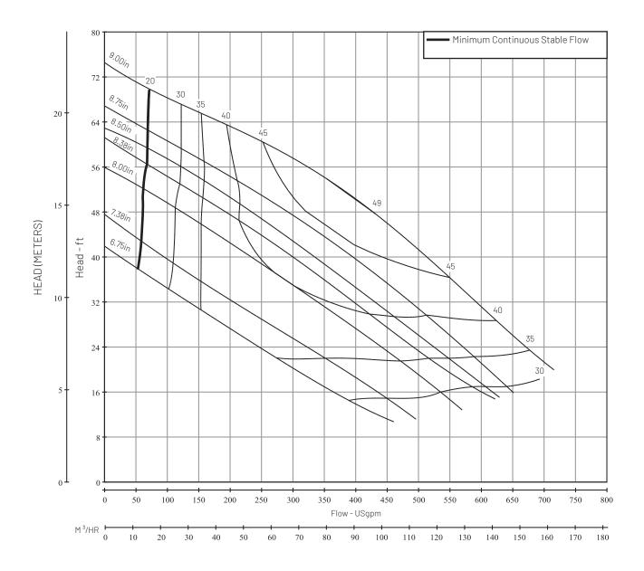
The curves reflect maximum performance characteristics without exceeding full load (Nameplate) horsepower. All pumps have a service factor of 1.2. Operation is recommended in the bounded area with operational point within the curve limit. Performance curves are based on actual tests with clear water at 70° F. and 1280 feet site elevation.
