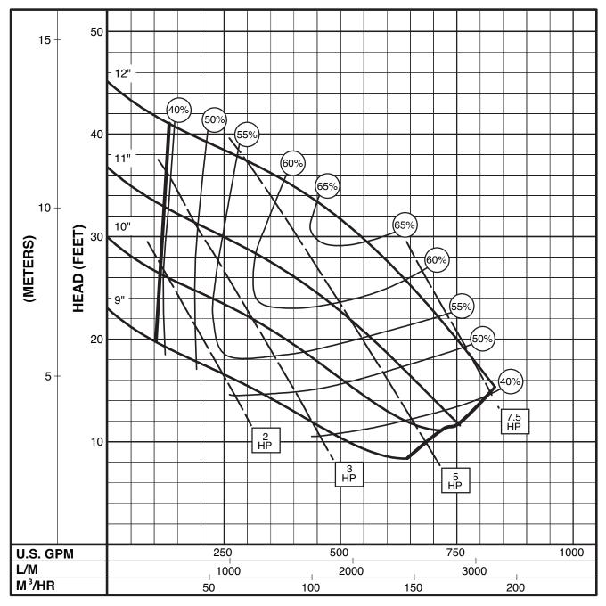
The curves reflect maximum performance characteristics without exceeding full load (Nameplate) horsepower. All pumps have a service factor of 1.2. Operation is recommended in the bounded area with operational point within the curve limit. Performance curves are based on actual tests with clear water at 70° F. and 1280 feet site elevation.
