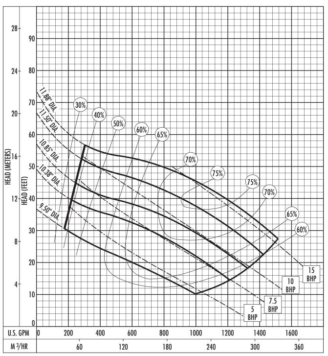
The curves reflect maximum performance characteristics without exceeding full load (Nameplate) horsepower. All pumps have a service factor of 1.2. Operation is recommended in the bounded area with operational point within the curve limit. Performance curves are based on actual tests with clear water at 70° F. and 1280 feet site elevation.
