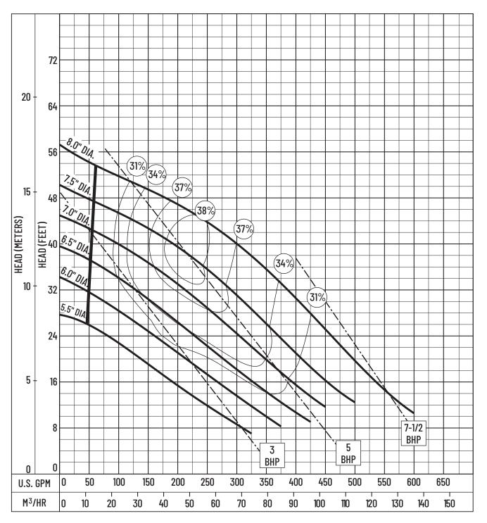
The curves reflect maximum performance characteristics without exceeding full load (Nameplate) horsepower. All pumps have a service factor of 1.2. Operation is recommended in the bounded area with operational point within the curve limit.
