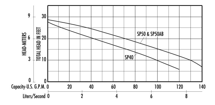
The curves reflect maximum performance characteristics without exceeding full load (Nameplate) horsepower. All pumps have a service factor of 1.2. Operation is recommended in the bounded area with operational point within the curve limit. Performance curves are based on actual tests with clear water at 70° F. and 1280 feet site elevation.
