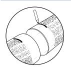
Mark the pipe ends to the proper minimum stab depth as appears in the product label.
