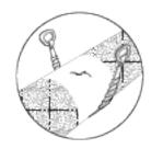
Prepare both pipe ends of the existing pipe by descaling if required. Clean the pipe as required using water. Make sure that the pipes are clear from debris and defects that may interfere with the HYMAX VERSA'S proper seal.
