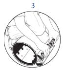
Once the HYMAX VERSA is around the pipe, engage the compression beam until it "clicks" into the 1st closing position (see below). The HYMAX VERSA can now be positioned over the leak covering the marks on both sides (see step 4).
