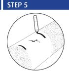
Mark the pipe evenly on both sides of the crack according to the length of the product.
