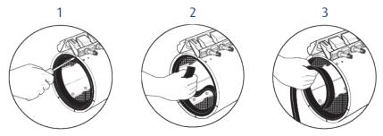
**NOTE: Measure the OD of the pipe TWICE using an OD tape!** Once the inner gasket is removed it can NOT be re-installed!
