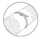
Measure the pipe's outer diameter and make sure the coupling's size will fit the pipe properly.
