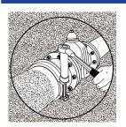
Tightening the end rings. Tighten the Flange Adaptor's bolts using a 3/4" socket wrench for 1.5"-3" Flange Adapters, a 7/8" socket wrench for 4"-12" Flange Adaptors, a 15/16" socket wrench for 14"-24" Flange Adaptors, and a 1.5" socket wrench for 26"-60" Flange Adaptors. Tighten the bolts evenly on each end ring in an alternating pattern to the torque mentioned on the label. Cross-tightening ensures that the gasket is evenly seated. When you finish, re-check the torque again.
