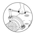
Tighten the end rings using a torque wrench, to the correct torque shown on the product's label. By tightening bolts the GRIP Elbow is steadily stabbed on the pipe.
