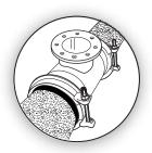
Position the Coupling for installation. If possible place the coupling(s) on the replacement pipe (on both ends) with top-facing bolts and lower the pipe and couplings into the ditch. Slide the couplings outward so that it covers the marks made in step 4.
