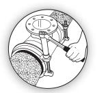
Tighten the coupling bolts to the right torque shown on the product label. When you finish, re-check the torque again.
