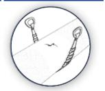
Prepare both pipe ends of the existing pipe by descaling if required. Clean the pipe as required using water. Make sure that the pipes are clear from debris and defects that may interfere with the HYMAX2 Outlet's proper seal.
