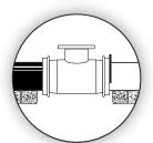
**NOTE:** HYMAX is not designed to support the weight of the pipes by itself. For uncoated ductile iron, grey cast iron and asbestos cement pipe surfaces - appropriate water-based gasket lubricant is required on both gaskets inside surface and pipe's outer surface.
