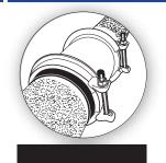
Position the coupling for installation. If possible place the couplings on the replacement pipe with top-facing bolts and lower the pipe and couplings into the ditch. Slide the couplings outward so that it covers the marks made in step 3. Make sure that the pipes are not touching inside the body of the HYMAX. There must be space between the pipes in order for continuous dynamic deflection to take place.
