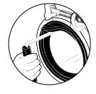
For size 1.5" only - use a lever (provided with product) to flip the gasket out if wider pipe diameter is required.
