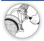
Tighten the end rings. Tighten the coupling bolts to the right torque shown on the product's label. When you finish, re-check the torque again.
