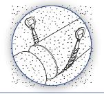
Prepare both pipe ends of the existing pipe by descaling if required. Clean the pipe using water. Make sure that the pipe is clear from debris and defects that may interfere with the HYMAX's proper seal.
