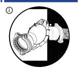
Installation: Slide the SWIVELJOINT on one pipe (Drawing 1) - do not tighten bolts. Position it so that it covers the marks made in step 4.
