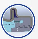
Unique dual sealing: In addition to the mechanical sealing, HYMAX Large Diameter achieves hydraulic sealing via its patented gasket that self-inflates using flowing water pressure.
