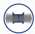
HYMAX's hydraulic sealing enables 4º continuous dynamic deflection per side, which substantially reduces future pipe breaks.
