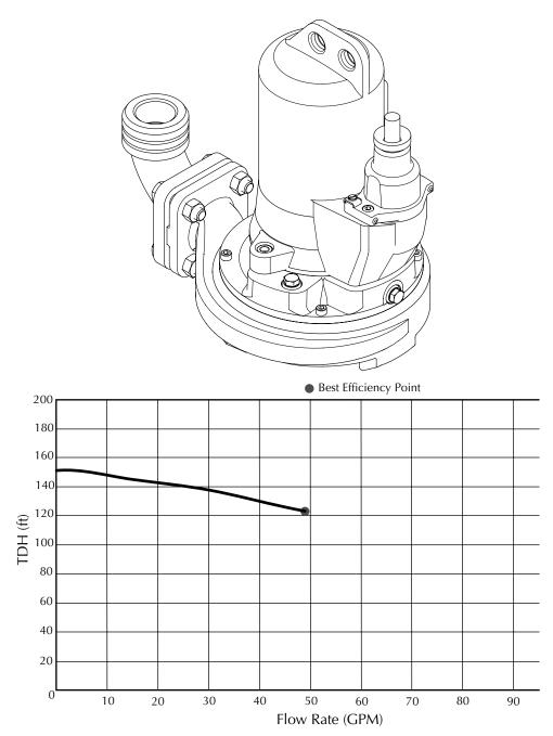
The curve reflects maximum performance characteristics without exceeding full load (Nameplate) horsepower. Operation is recommended near the Best Efficiency Point. Operating at the outer limits of the curve is not recommended. Performance curves are based on actual tests with clear water at 70° F. and 1280 feet site elevation.
