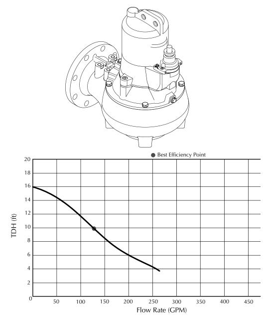
The curve reflects maximum performance characteristics without exceeding full load (Nameplate) horsepower. Operation is recommended near the Best Efficiency Point. Operating at the outer limits of the curve is not recommended. Performance curves are based on actual tests with clear water at 70° F. and 1280 feet site elevation.
