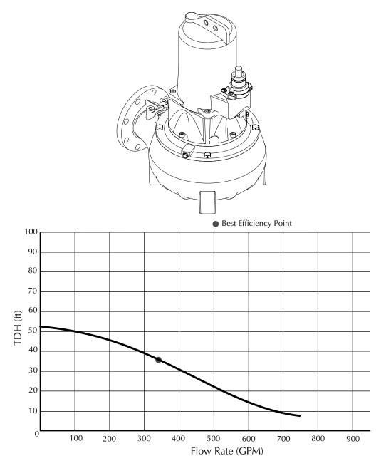
The curve reflects maximum performance characteristics without exceeding full load (Nameplate) horsepower. Operation is recommended near the Best Efficiency Point. Operating at the outer limits of the curve is not recommended. Performance curves are based on actual tests with clear water at 70° F. and 1280 feet site elevation.
