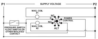
TYPICAL WIRING DIAGRAM FOR THE ALT-X (CROSS CONNECTED)
