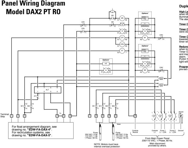
when lifted. The audible alarm may be silenced by pressing the illuminated PUSH TO SILENCE button on the front of the control panel The alarm light will remain on until the float is lowered.
