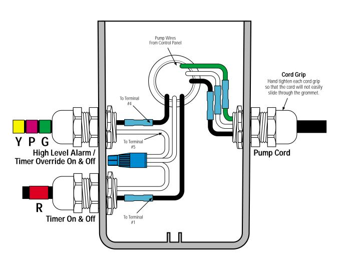
Key Black Wire White Wire Green Wire Waterproof Wire Nut Heat Shrink & Butt Connector \*
