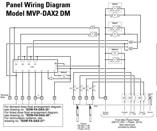
NOTE: Motors must have internal overload protection
