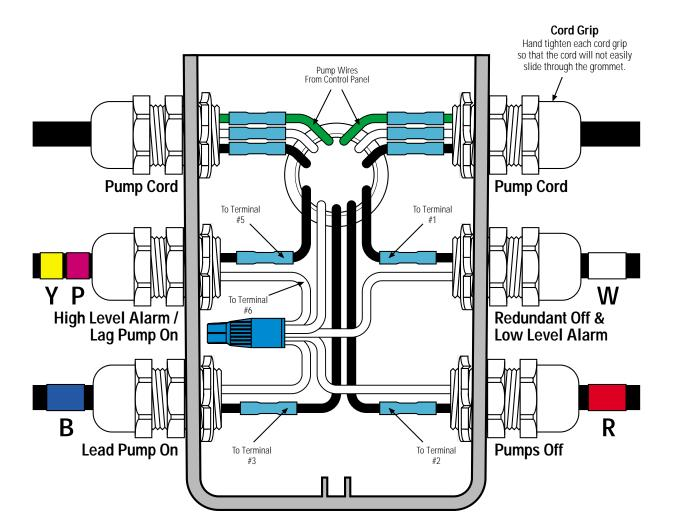
Key Black Wire White Wire Green Wire Waterproof Wire Nut Heat Shrink & Butt Connector \*
